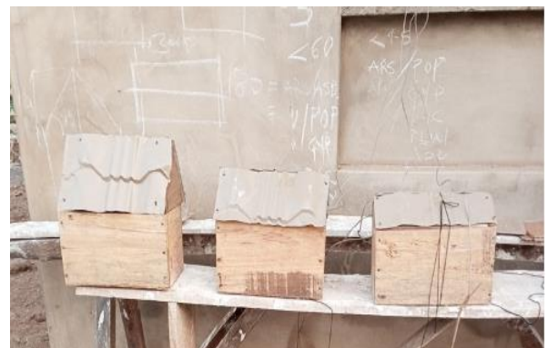
Plate 3: Experimental set up for aluminium roofing sheet with selected ceiling materials
