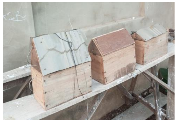
Plate 2: Experimental set up for plywood-lined aluminium roofing sheet with selected ceiling materials
